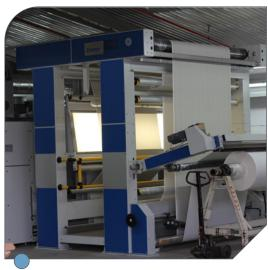
10 | Various fabric exit devices or smooth and reliable web guiding at any speed. Plaiter with e.g. J-Box, antistatic devices, inspection table or center winder.
