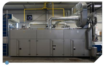
**9** | **The COMPACT.HC dryer** with an operating temperature of 90°C to 200°C is available on ground floor level or elevated on a substructure. With optimized interior geometry for high energy efficiency and uniform chamber temperature. Self-monitoring and state-of-the-art measuring and regulation techniques.
