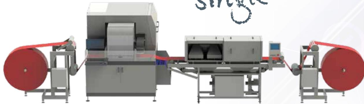
The COLARIS-NF Single is a single-pass digital printer for one-sided printing on narrow fabrics. One-sided printing is typical for individualizing consumables such as face masks or cleaning wipes. It is also used for printing on hook & loop quick-fix-and-release tapes, bandages or decorative tapes.
