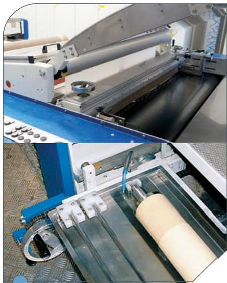
**4 | Wet glueing device** with optimized squeegee application system and automatic glue feeding pump.
