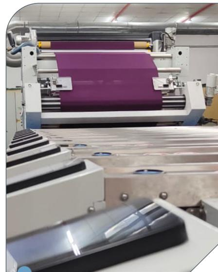
**3 | The high quality lattice roller** in combination with soft air blowing edge uncurlers assures tensionless transport from the roll or trolley onto the printing blanket.
