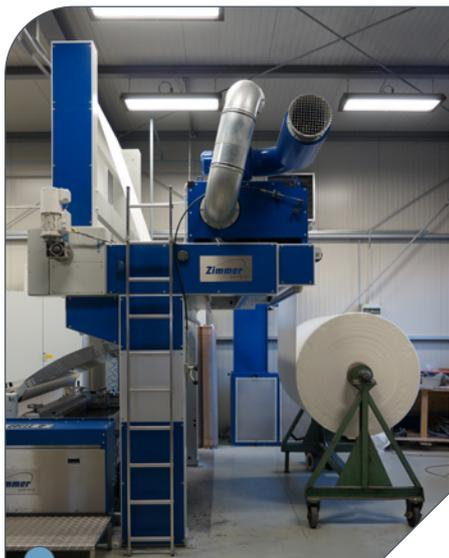
**1 | The unbatching device** comes with a stepless automatic digitally controlled speed control drive system, which transports any kind of woven and knits from small or large rolls onto the printing machine.
