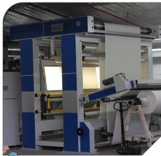
**10 | Various fabric exit devices** or smooth and reliable web guiding at any speed. Plaiter with e.g. J-Box, antistatic devices, inspection table or center winder.
