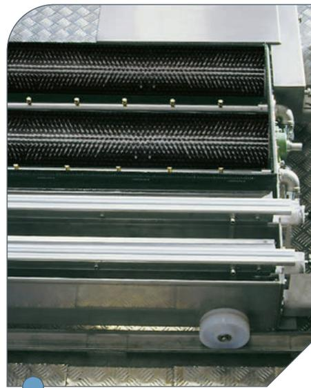
**8 | Printing blanket washing device** with high quality brushes and water recycling system for a minimum of fresh water consumption.
