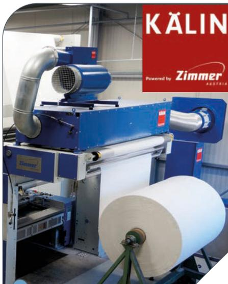
**2 | Dust and lint removal device** new and improved, for most efficient fabric cleaning results. The standard basic suction system optionally can be combined with a brushing, blowing or beating system. One-side or both-side cleaning may also be opted.
