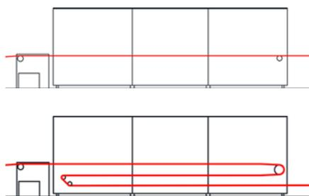
The modular construction of this high efficiency hot air dryer with conveyor belt can be designed with one, three, or up to seven passages for higher productivity. Especially for thick permeable substrates such as coated and wet textiles or nonwovens.
