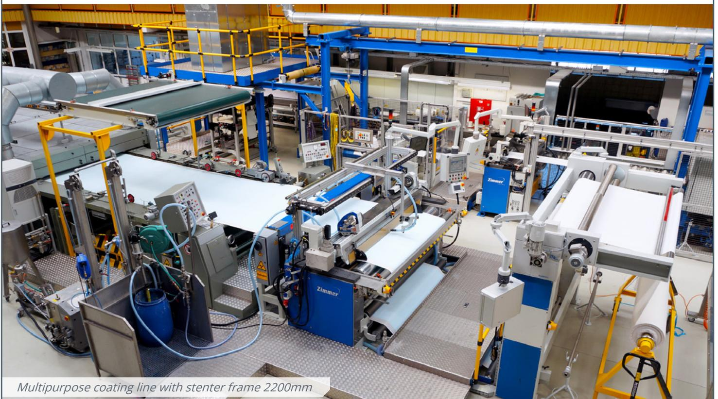
*Multipurpose coating line with stenter frame 2200mm*
