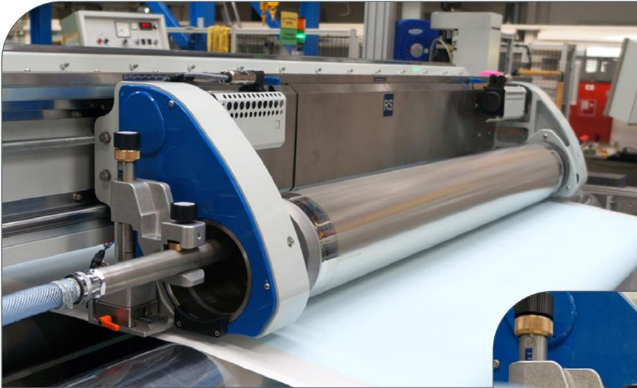
MAGNOROLL coating machine with screen coating module
