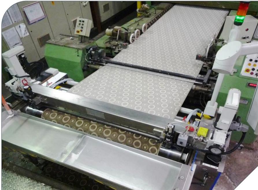
MAGNOJET foam coating unit installed in stenter frame line
