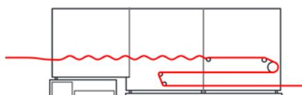
Lay-on-air floating fabric guiding in the entry zone of the dryer, combined with a conveyor belt. Lay-on-air-nozzles for contact-free surface drying, especially for fully penetrated fabrics.
